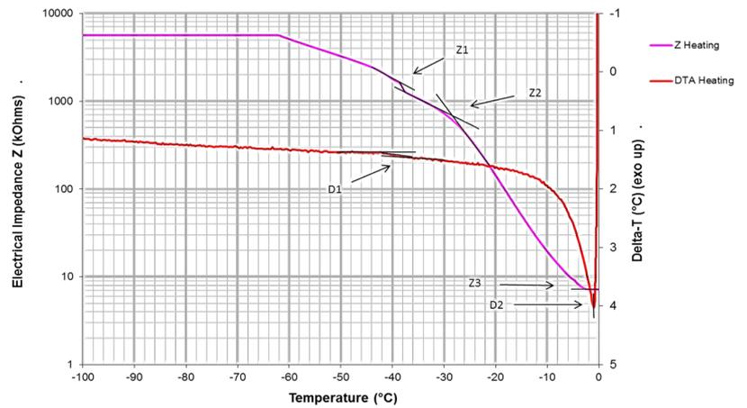
**Figure 2:** Lyotherm3 graph showing events in DTA curve (in red) and impedance curve (in pink)
