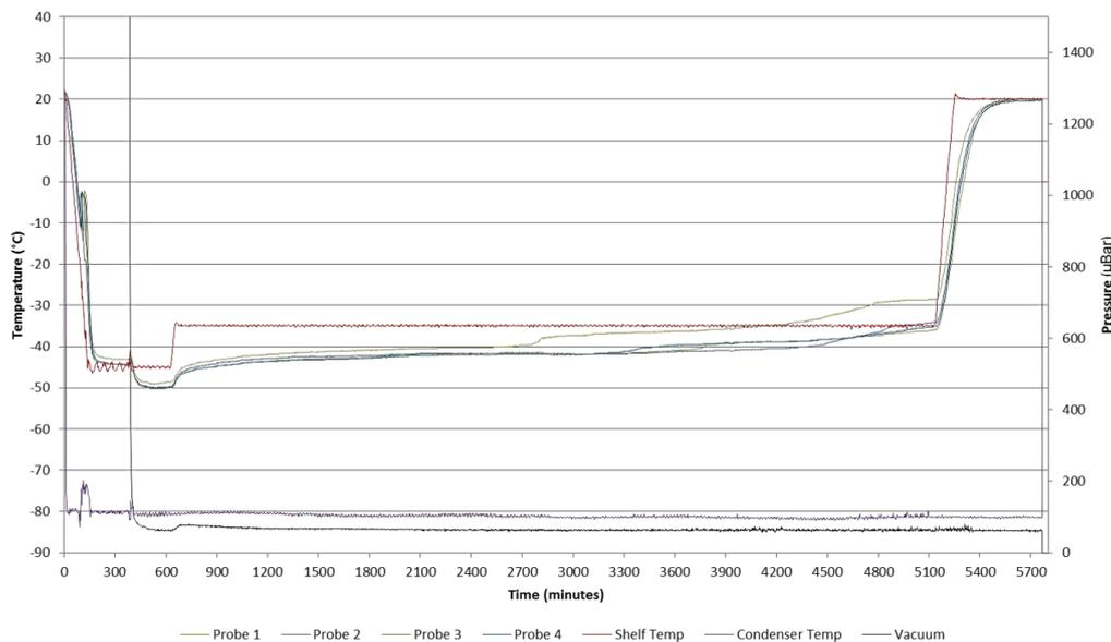
**Figure 3:** Final (96 hour) freeze-drying cycle for ADC
