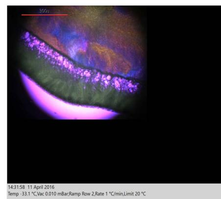
Figure 1: FDM image of formulation at  $-33.1^{\circ}\text{C}$
